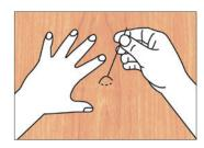
If during installation air should be trapped behind the film causing a bubble, gently strip back the film and reapply with the plastic applicator. Very small air bubbles can be released by pricking the bubble with a pin. Press out the entrapped air by moving your thumb toward the puncture.
