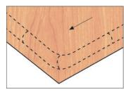
Cut the film 100mm larger than the substrate size.
