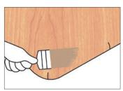
Once any bullnose or curved edges have been shaped and sanded, apply primer to the curved surface and reverse side.
