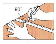
Place a ruler on the center of the joint. Carefully slice through both pieces of the film. The knife blade should be at right angles to the film.
