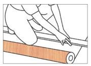
Lay the film on flat working table and measure the substrate. Always cut the film allowing for a 2~4cm over trim.
