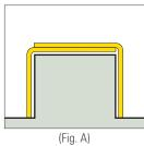
Apply the film by overlapping both sides on the joint at the top of the door.
